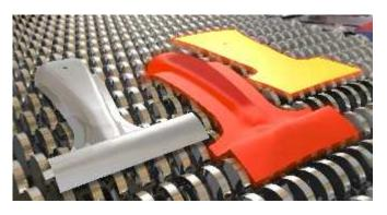
With this plug-in, the user can also simulate the tailored tempering process, thus enabling the engineering of stamped parts with targeted local strength properties. Based on the results of AutoForm-PhaseChange plug-in, crash simulation accuracy can be improved by taking into account the real strength distribution of the hot-formed component.
