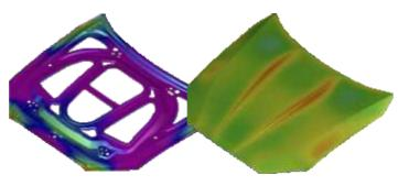
New Target for Hood Inner after Compensation
