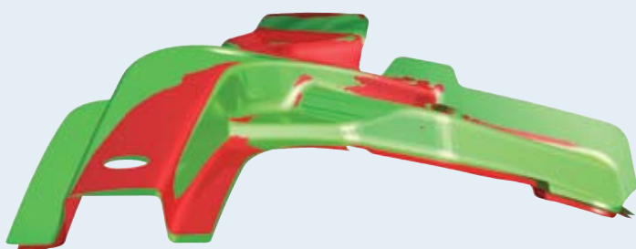
The compensated tool geometry of a first simulation is used as input for the next simulation. After several compensation loops, springback is within the required tolerance. Comparison of part geometry (red) to reference geometry (green) before springback compensation (left) and after compensation (right).
